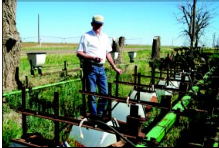
This hooded sprayer was designed and built by Don Mimms for his conservation tillage operation.
